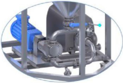
Powder and liquid are strongly sucked into the pump chamber
